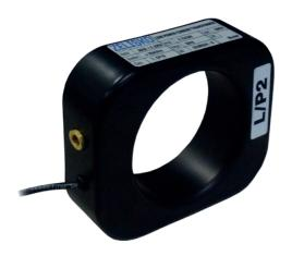
This type is designed for simple original equipment in switchgears. It is slide on the not mounted output T-connector in the substation. When the connector is screwed on the feed through, its sheathing expands. Thus, the sheathing presses against the inner surface of the current sensor and fixes it. Consequently, additional fixations of the sensor in the substation are not necessary.
