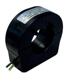
The retrofit application in existing installations is the primary field of application for this type. The click system enables a tool-free mounting of the sensor on site. Dismounting of the T-connector is not necessary, since the sensor is enclosing the cable.
